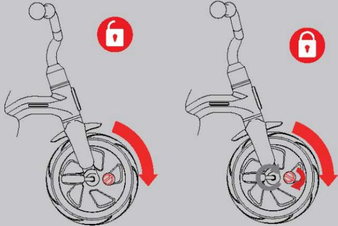
Note: When push mode, the front wheel should be adjusted to leave mode.
